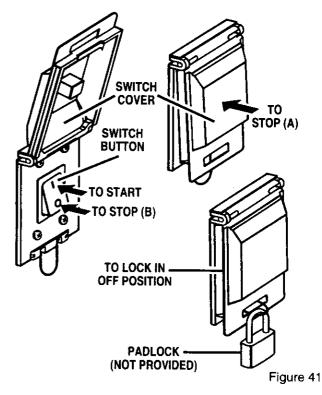
■ To turn saw Off, (A) press or push outside of switch cover, or (B) lift switch cover and press switch button. See Figure 41.
